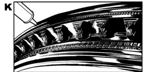
Apply paintable caulk to edges
