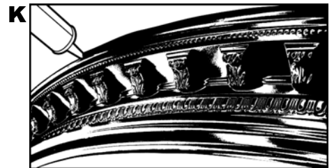
Apply paintable caulk to edges
